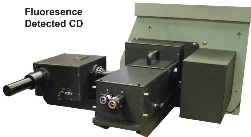
Emission monochromator addition with digital photon counting detector.
