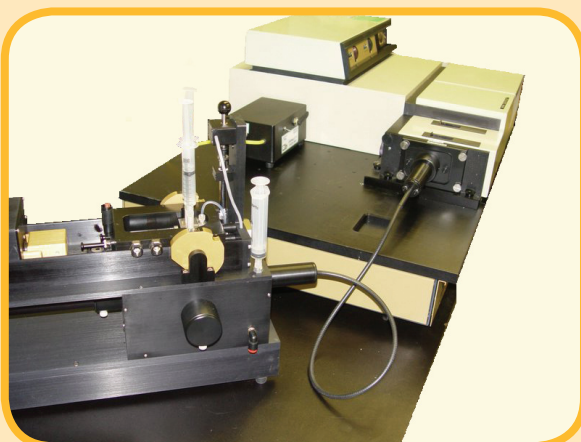
Light guide attached Olis USA stopped-flow to an Aminco DW-2
